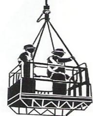
**Personal Fall Arrest System** – means a system to arrest an employee in a fall from a working level. The system consists of an anchorage, body harness, connectors, lanyard, deceleration device, lifeline, or any suitable combination of these. The use of a body belt for fall arrest is prohibited.
